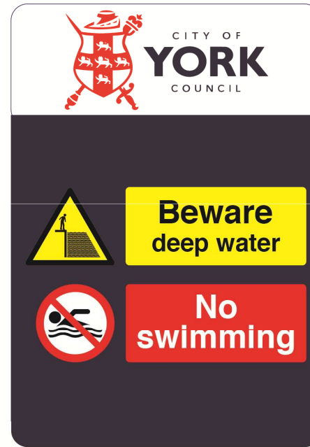
30 (no) 210 x 300mm Aluminium Composite Material signs with riveted channels to rear
